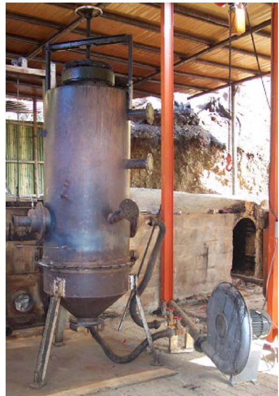
Fig. 3. Snapshot of the constructed updraft fixed bed gasifier with an embedded combustor.
